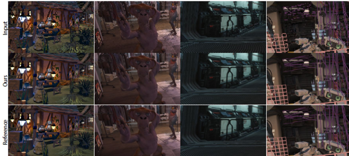
Fig. 1. Results of our real-time, learned 4 \times 4 supersampling are shown for four sample scenes. From top to bottom: the rendered low-resolution color input, our reconstruction, and the rendered reference images. Our supersampling method takes the color, depth, and motion vectors of multiple low-resolution frames, and produces high-fidelity reconstructions by reducing aliasing and recovering scene details.
