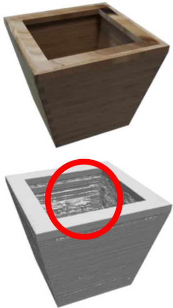
Imperfect shape surface (Non-manifold, non-watertight)
