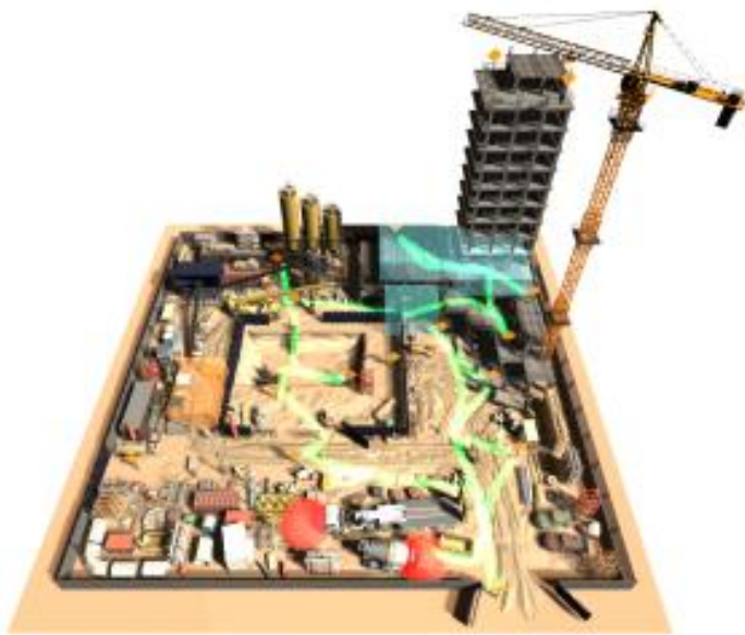
(b) Synthesized route with more fall hazards.
