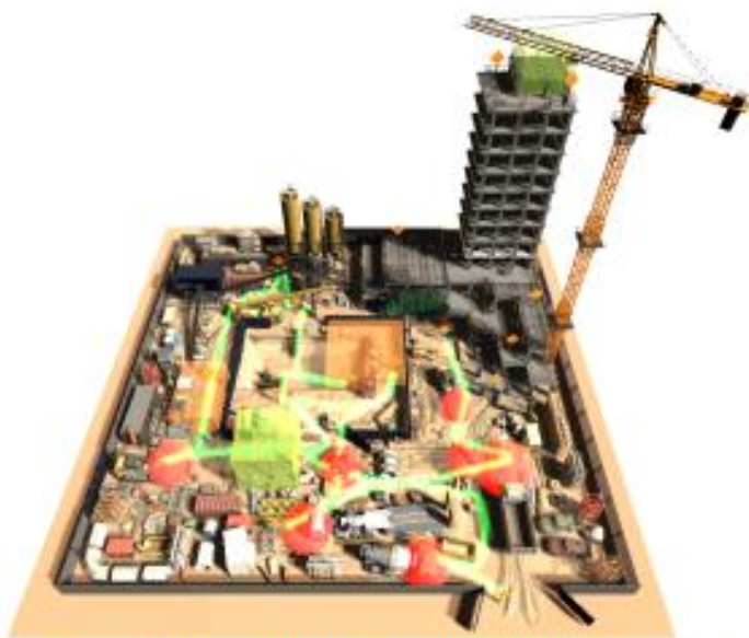
(e) Synthesized route with more struck-by hazards.
